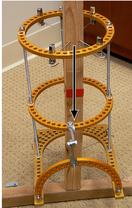
Fig. 3. Biomechanical loading pattern applied with a circular ring external fixator. The biomechanical load is applied via a force vector through the center of the bone, without a bending moment about the fracture/osteotomy site.
