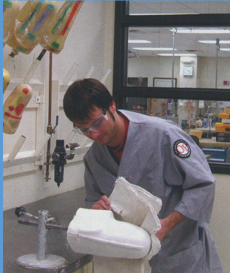
MODIFYING MODEL to create posterior brim for quadrilateral socket
