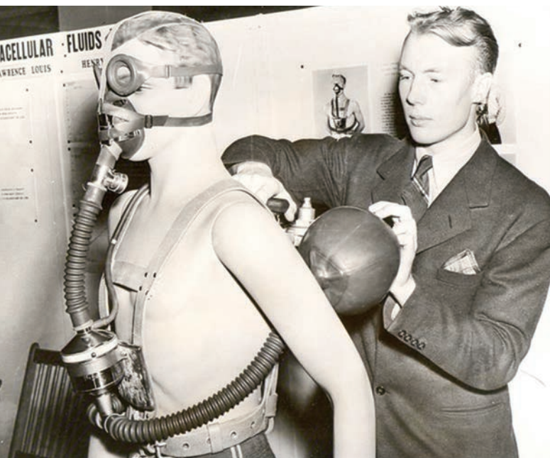
While a Penn medical student, Christian J. Lambertsen (M 1943), an expert on respiratory physiology, invented the Lambertsen Amphibious Respirator Unit, or LARU, forerunner of today's scuba technology.
